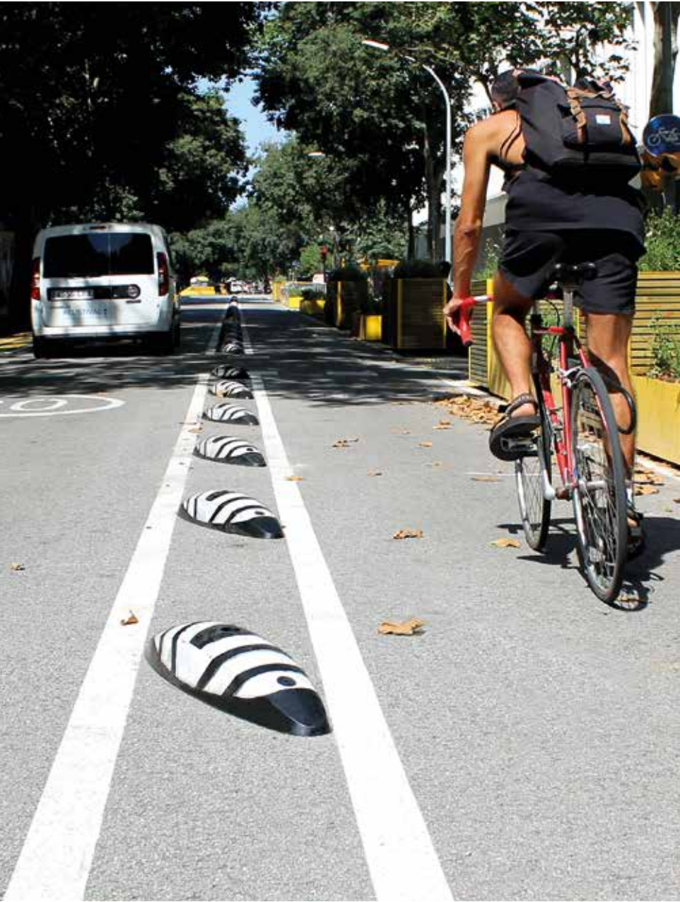
Separator Gota VBA21 748 x 50 x 50mm 775 x 164 x 90mm 820 x 210 x 130mm
